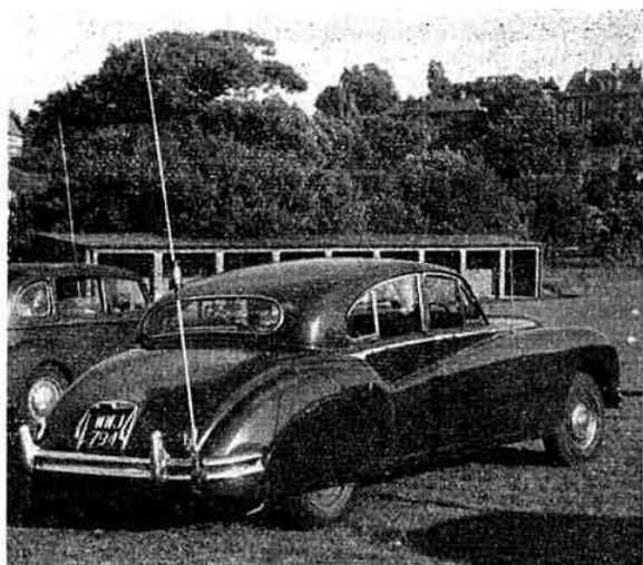
Centre loaded whip mounted on G5CP's car.
